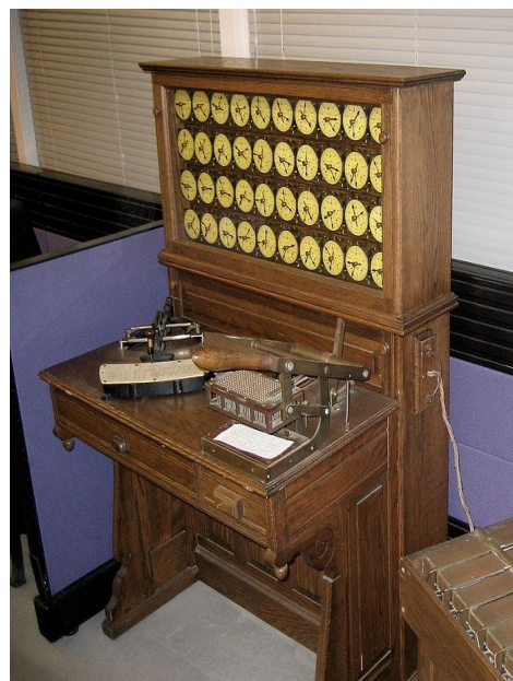
Hollerith Tabulation Machine with sorting box visible on right. Source: Wikipedia
